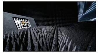
▲ Fig. 1 OTA test chambers are needed to test highly integrated mmWave components, which often lack physical connections.
