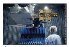
Fig. 1 Testing an antenna system integrated on a satellite. Source: ESA.
