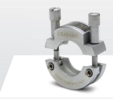
The waveguide quick connect is used to connect and disconnect mating flanges of waveguides efficiently and reliably without any complications. It uses thumb screws to effortlessly clamp two flanges together to create a perfect connection for two mating waveguides that eliminates tedious waveguide screw alignments to avoid signal leakage and impedance mismatch due to waveguide mating misalignment.
