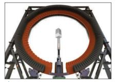
★ Fig. 2 SG Evo multi-probe, spherical, near-field antenna measurement system.
